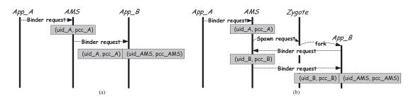
Fig. 3. Binder IPC Propagating Diagram in Component Interaction from App\_A to App\_B. (a) When App\_B is started. (b) When App\_B is not started.
