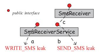
Fig. 10. Permission leak paths in Mms application.
